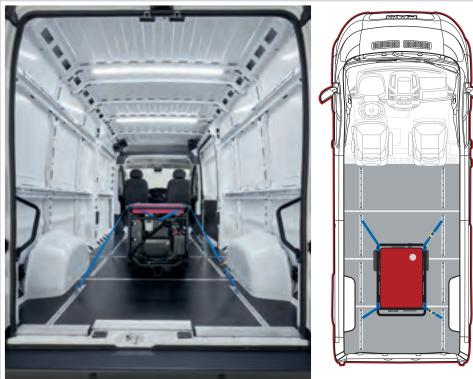
**CARGO TIE-DOWN TRACK SYSTEM.** This is multitasking at its best. The load floor system includes two in-floor tracks and two side tracks—one on each wall. Fitting all tracks are four 5/16-inch carriage bolts and four L-Channel Quick-Connect rings to securely strap down cargo—and they all work with the available shelving units as well. (Straps not included.)
