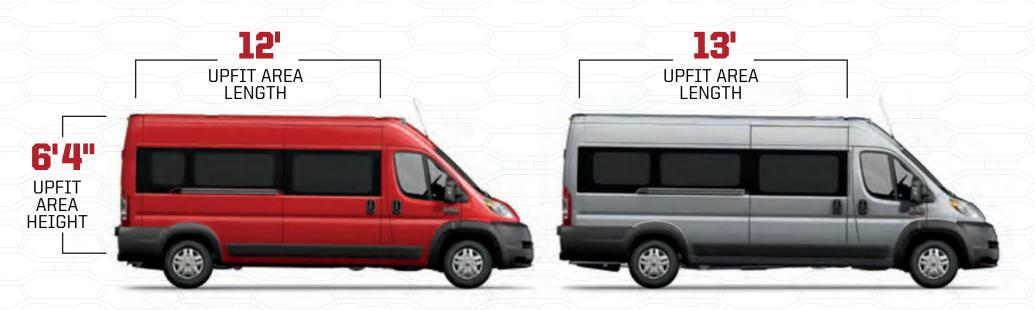
**ONE WHEELBASE, EXPANSIVE OPTIONS.** Utilize the extended body on Windowed Van to create a significantly larger interior. The 14.4-inch extension adds nearly 43 cubic feet of volume-the perfect solution when you need extra room for luggage or storage.
