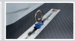
**THE CARGO LOAD FLOOR: MODULAR AND THE PERFECT FIT.** Available at the time of initial order and installed at the factory, the Mopar Cargo Load Floor includes multiple floor and wall tracks (A) with hardware, a non-slip surface and convenient angled leading edges (B) to make loading and unloading a breeze.
