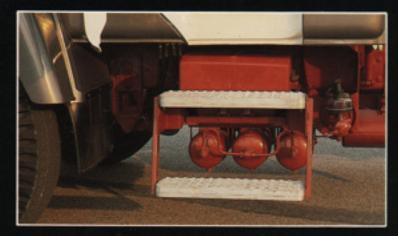
Low cab height, wide door openings, strategically placed self-cleaning cab steps and grab handles make entry/exit safe and easy. The CS200 air over hydraulic brake system components are mounted under the cab, leaving a clear platform for a wide variety of body configurations.
