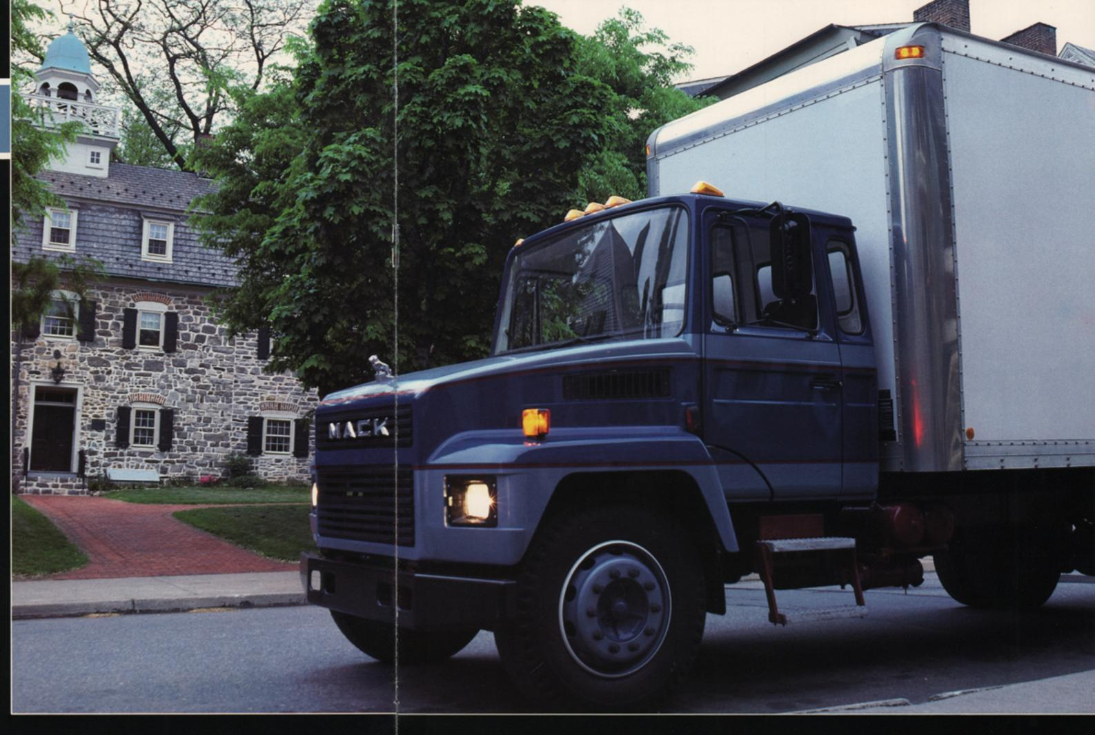
The Mid-Liner CS grille panels are interchangeable for easy replacement. Behind the grille, a sealed junction box with wiring in loom protects lamp connections.
