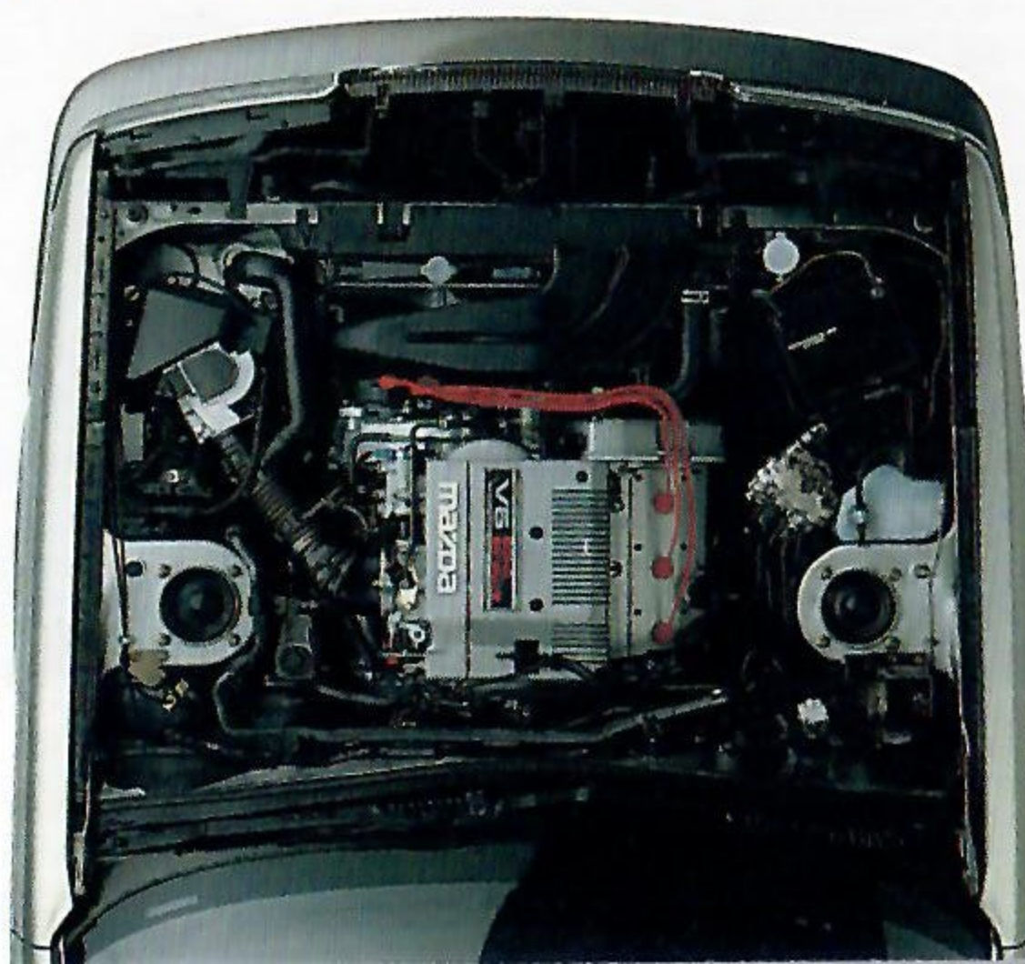
The 929S 3.0-liter DOHC 24-valve V6.
