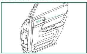
Inside rear door handles are disconnected. Rear doors can only be opened from the outside.
