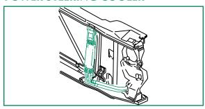
Vertical finned cooler is mounted at the left end of the radiator and connected in-line between the power steering pump and steering pump and steering gear.
