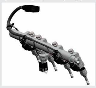
With direct injection, fuel is sprayed directly into the engine cylinders, where it is mixed with air. The gasoline/air mixture cools the cylinder, allowing the engine to make more power. In general, an SIDI engine produces more power than a port-injected engine of similar displacement and design.
