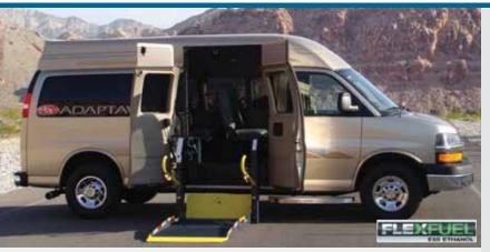
Chevrolet Express Cargo is the full-size van of choice for mobility applications. The Express Cargo Paratransit (Y3H) is offered in 2500 and 3500 models, in regular or extended wheelbases. Express Cargo is a practical choice for installing adaptive equipment and mobility accessories, such as wheelchair lifts, ramps, running boards, and driver aids, available from independent aftermarket suppliers.
