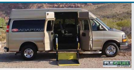
GMC Savana Cargo is the full-size van of choice for mobility applications. The Savana Cargo Paratransit (Y3H) is offered in 2500 and 3500 models, in regular or extended wheelbases. Savana Cargo is a practical choice for installing adaptive equipment and mobility accessories, such as wheelchair lifts, ramps, running boards, and driver aids, available from independent aftermarket suppliers.
