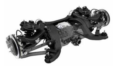
Standard on V8 models and on V6 manual models, a limitedslip differential helps to improve traction by directing engine power to the rear wheel with the best traction. This gets the power to the ground for enhanced performance, especially in low-speed corners and low-traction conditions.
