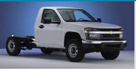
Chevrolet Colorado Chassis Cab gives commercial truck buyers a solid platform to meet their vocational needs. Instead of a pickup box, the chassis cab model allows specific boxes or platforms to be installed by a third-party source.
