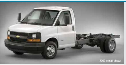
The G4500 has a 14,200-pound GVWR<sup>5</sup> and 4,600-pound front GAWR. That makes for a best-in-class payload (class 4). To accomplish this, heavy duty chassis components and reinforcements are used, and a different rear axle and frame is used versus the 3500 cutaway.
