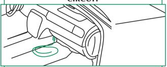
Two 16-gauge wires are connected to an in-line connector in the horn circuit of the instrument panel harness under the instrument panel. The end of this harness extension is terminated with an in-line connector in a 60-inch coil under the instrument panel. Connection to customer switching permits operation of the horn or siren with the horn button.
