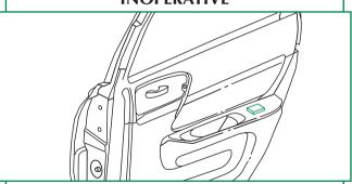
Rear door window switches are inoperable. Rear door power regulators are operable only from driver position switches.
