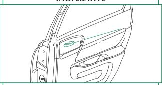
Rear door locking rods are disabled. Rear door locks are inoperable at rear doors, but operate from driver position.
