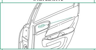
Inside rear door handles are disconnected. Rear doors can only be opened from the outside.
