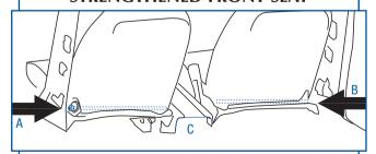
Seat bottom frame structural tubes - A,  $\,$ B Center floor tunnel-mounted crush box -  $\,$ C
