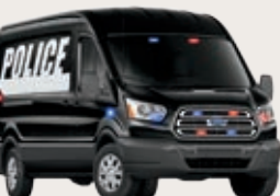
Transit Prisoner Transport Vehicle¹ 31.1, 32.1, 34.1 (3.7L Ti-VCT V6 standard; 3.5L EcoBoost V6 optional; 3.2L Power Stroke® I-5 Turbo Diesel optional)
