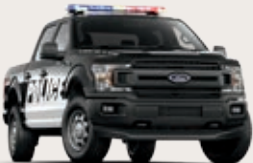
F-150 Special Service Vehicle 50C.1, 55C.1 (5.0L Ti-VCT V8 FFV standard; 3.5L EcoBoost V6 optional)
