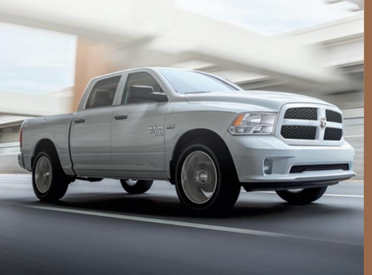
**TOUGH FRAME** If you're going to build on anything, build on strength. In the case of Ram 1500 Classic, we're talking high-strength steel core, eight ultratough crossmembers and a hydroformed tubular high-strength steel front frame unit.
