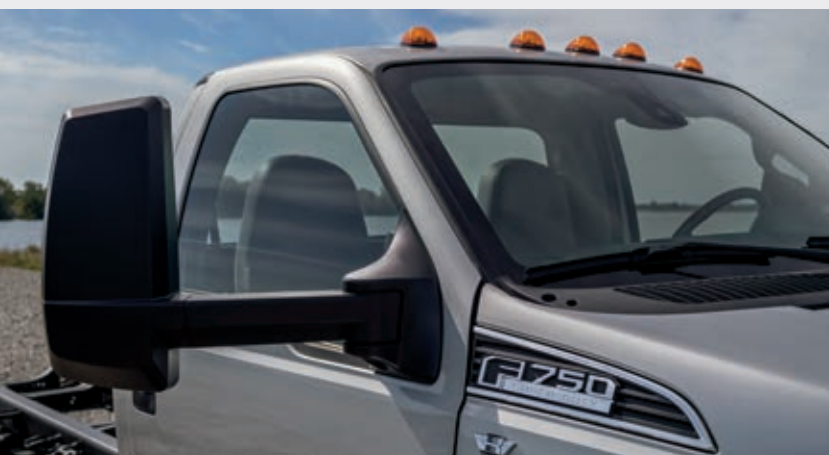
Dual manual-folding, heated, sail-type mirrors include integrated spotter mirrors and can reach up to 102" wide Available
