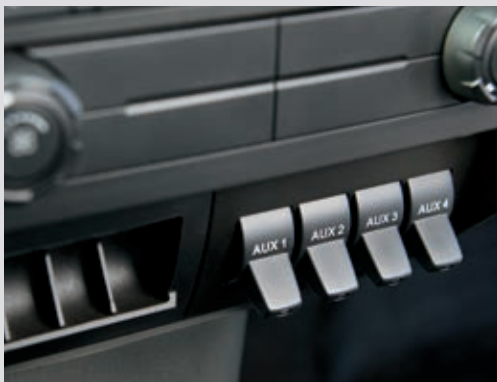
Standard upfitter switches on diesel
