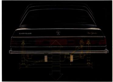
**Automatic load-leveling** rear suspension option adjusts suspension height to compensate for variations in the weight of passengers and luggage.
