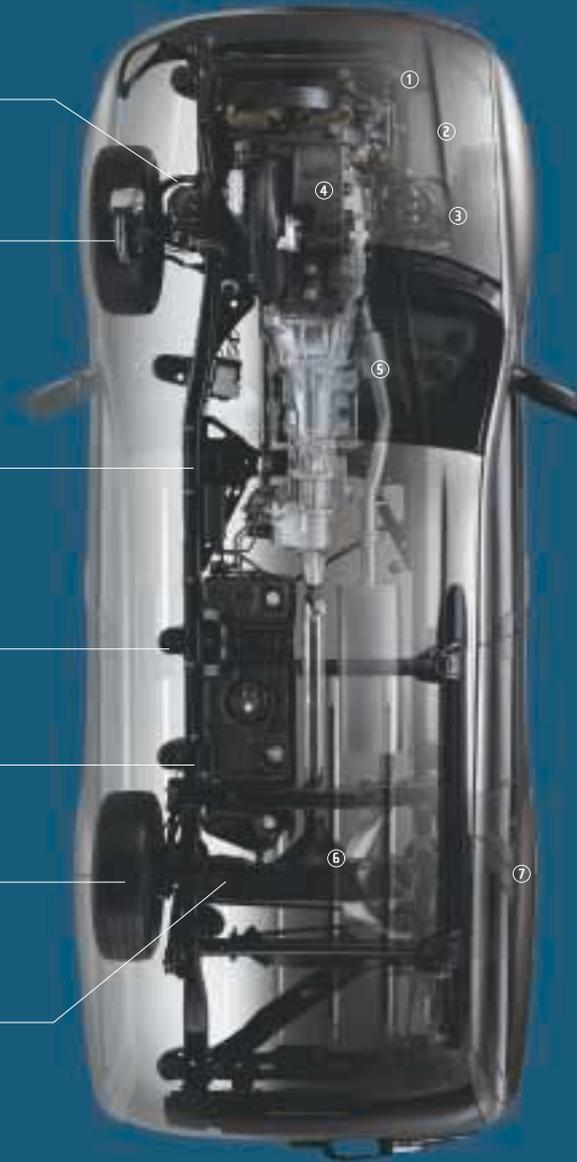
1. To create the best fit and maximum rigidity, the radiator support and structural cross members are welded together prior to installation on the frame.
