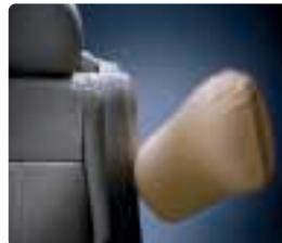
The standard dual frontal air bags are complemented by driver and front-passenger side-impact air bags to provide an added level of occupant protection in a moderate to severe side impact collision.
