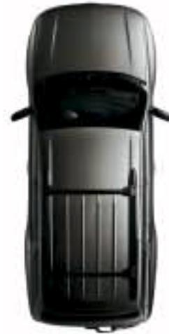
The integrated design of the standard rooftop luggage rack blends seamlessly into the overall exterior styling. The rack can carry up to 200 lbs of cargo. For added convenience, you can opt for an accessory bicycle carrier.\*
