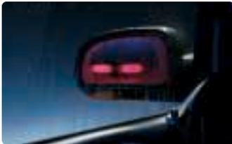
The outside rearview mirrors are boldly styled and have a standard defogger to enhance visibility. They also have available turn indicators, a memory recall and an Electrochromic feature on the driver's side that automatically reduces distracting glare.
