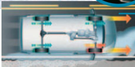
Available on Safari and Savana 1500, all-wheel drive (AWD) helps keep you from getting stuck by sensing when a wheel is starting to slip and automatically redistributing torque to the wheels with superior traction.
