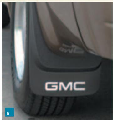
a. Splash guards – Made from fortified, rubber-reinforced polypropylene. Various styles available.
