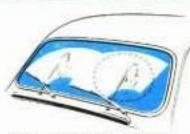
The windshield wipers cover large, intersecting zones. They are operated by the same control as the washers. Flying stones cannot hazard visibility - the windshield includes a special emergency "see-square".
