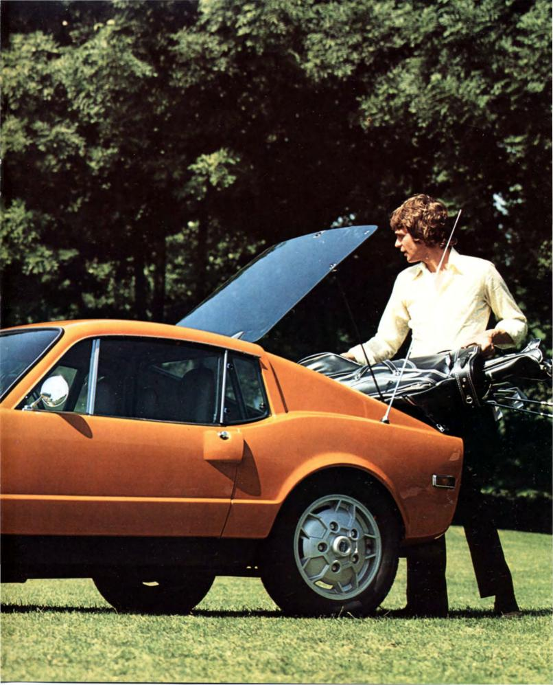
There are lots of other Sonett features that are equally easy to appreciate like a 4 speed shift on the floor, molded bucket seats, a leather covered steering wheel, front wheel disc brakes and full instrumentation. Plus the fact that Sonett has roll bars both in the windshield pillars and behind the seats.
