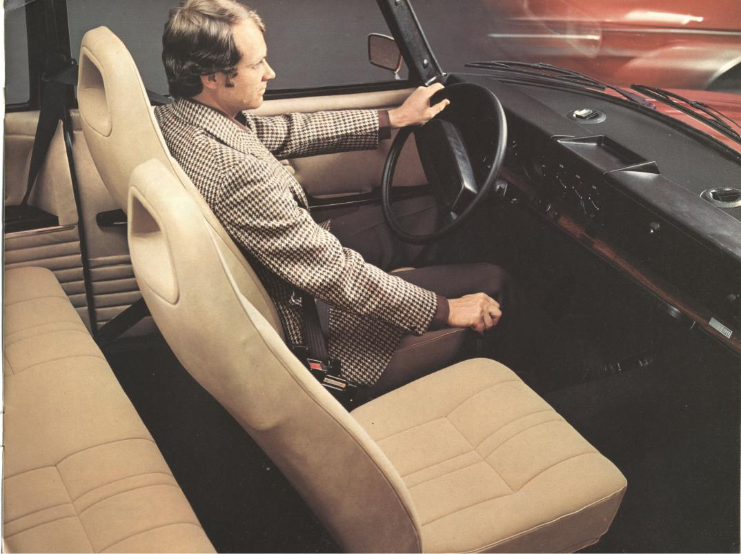
The height of the seat cushion can be easily adjusted and it can be inclined to suit individual requirements. The front to rear adjust is almost as much as six inches (160 mm).
