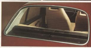
The rear window is kept continuously clear of mist by the warm air defroster. For quick defrosting, the rear window is also equipped with an electric defroster.
