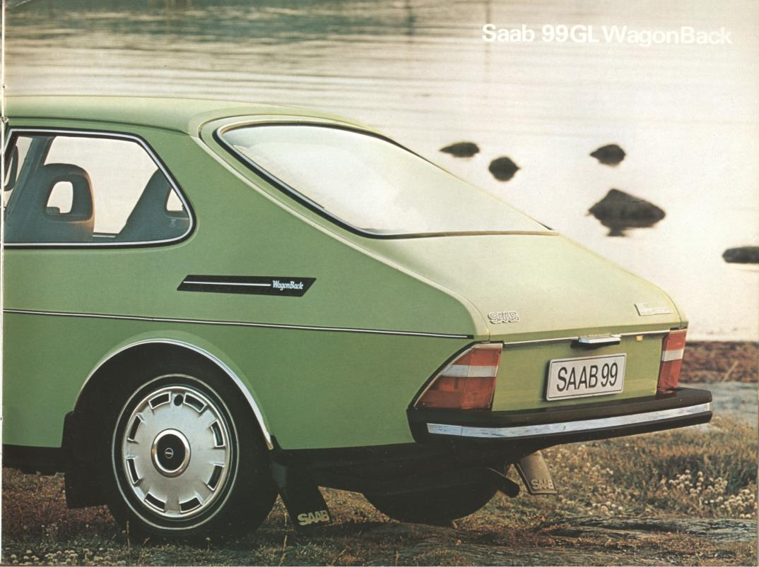
The floor of the WagonBack is only 21 inches (53 cm) off the ground so it's easy to lift things into the back. And the rubber covered bumper provides a practical support when loading heavy items.
