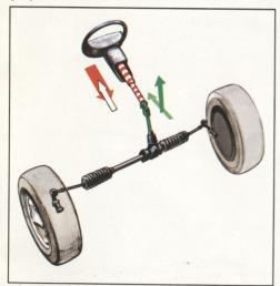
steering column is jointed and telescopically collapsible, making our rack-and-pinion steering system not only direct and precise, but safe, as well.
