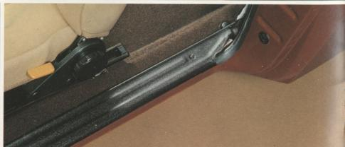
The sill beams are low and recessed to make entry and exit easy. The sill beams are protected from road dirt by the doors.
