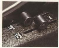
The rear doors are provided with child-proof locks—a latch makes it impossible to open the door from the inside, but not from the outside.
