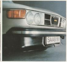
The Saab EMS has been equipped with a new front spoiler for improved gas mileage and handling.
