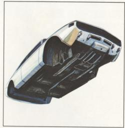
All welded seams and joints are placed as high as possible, out of the way of dirt and moisture. As additional moisture protection, all exposed joints are sealed off with a high quality, elastic sealing agent.
