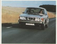
Every EMS has a fuelinjected 2-liter overhead cam engine with a fourspeed all-synchro gearbox, for the kind of performance a sports sedan should have.
