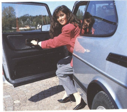
The doors have a wide opening angle. The sills are set back and protected against road dirt.
