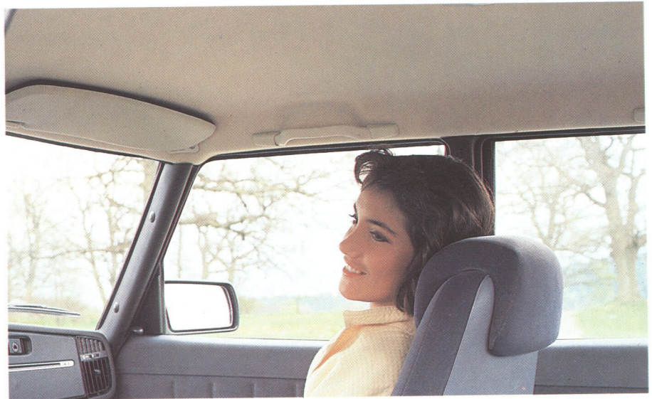
The moulded glass fiber roof lining is covered with velour and provides insulation against noise, heat and cold, as well as an impact-absorbing surface covering the roof and reinforcing members.
