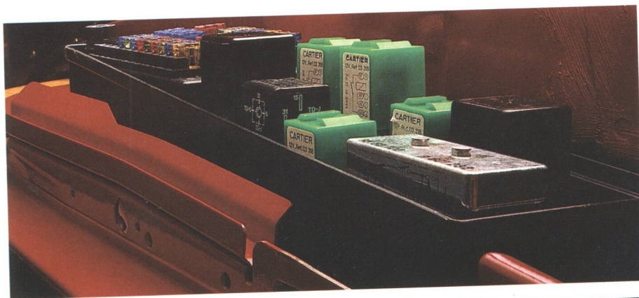
The fuse box is designed to accommodate 10 relays and 31 fuses, plus 7 spare fuses in separate holders.
