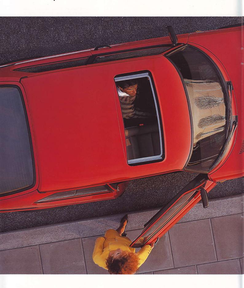
The deeply curved windshield improves aerodynamics, uses wind force to push rain, snow and dirt to the sides, and enhances safety by moving the glass farther forward from the front-seat occupants.
