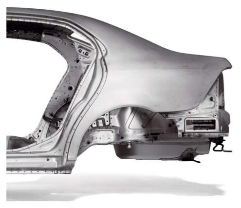
**Safety cage** – beams and high-tensile steel reinforcements around the passenger compartment. Front and rear crumple zones are designed to catch and distribute collision forces over a wide area to help reduce the effects of a collision on the car's occupants.
