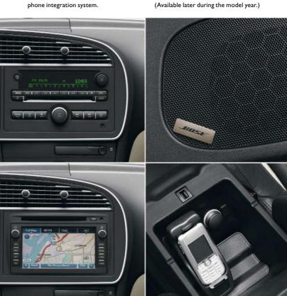
Saab Infotainment Plus – includes AM/FM stereo tuner with RDS, MP3-compatible CD player, 6.5" colour touchscreen and navigation. Voice-controlled. AUX connection for your MP3 player and other portable audio equipment. Can be combined with the Bluetooth™ phone integration system.
