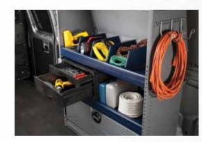
COMPOSITE SHELVING AND STORAGE REDUCES NOISE AND HELPS INCREASE FUEL EFFICIENCY
