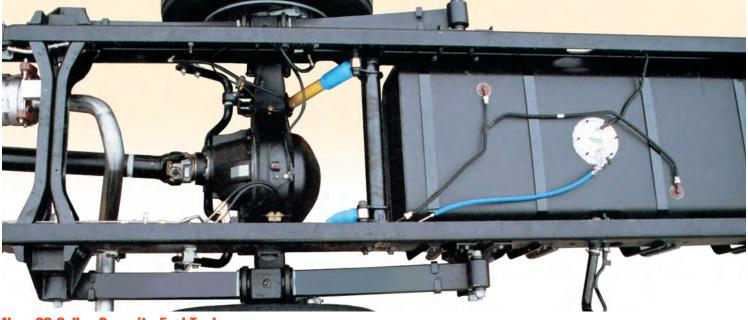
New 80-Gallon Capacity Fuel Tank The 2011 Ford Class A Chassis now features an 80-gallon (302-liter) capacity fuel tank for increased driving range. Integrated into the tank is a new fuel pump that includes a long-life fuel filter. This eliminates one item, and its associated expense, from the normal maintenance schedule.
