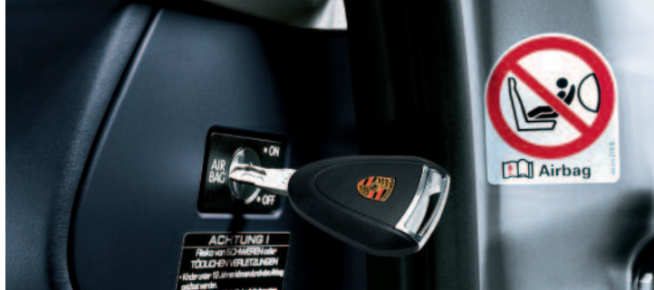
Deactivating the front-passenger airbag
