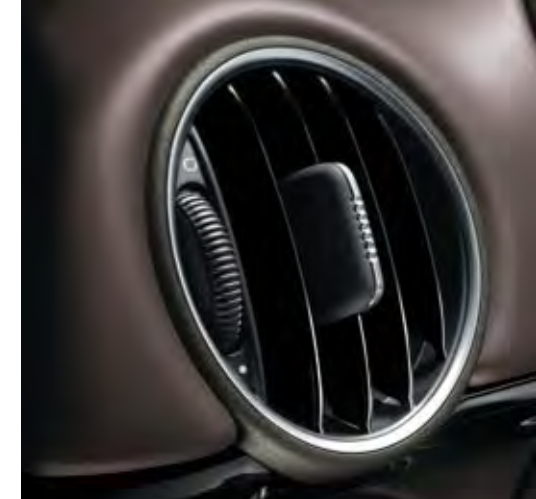
Air vent slats painted
