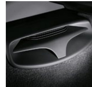
Active subwoofer, 4-inch x 6-inch (10.2cm x 15.3cm) bass speaker in the passenger footwell
