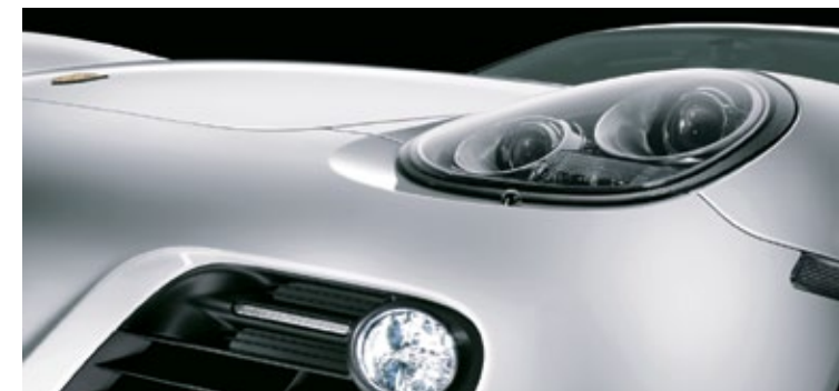
Bi-Xenon™ headlights with dynamic cornering lights and LED daytime running lights
