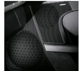
3-inch (8.0cm) neodymium mid-range speaker and 8-inch (20.0cm) Nd 1 bass speaker
