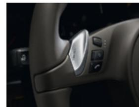
PDK gearshift switches on multifunction steering wheel
