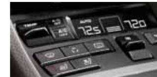
Seat heating, seat ventilation, two-zone automatic climate control
