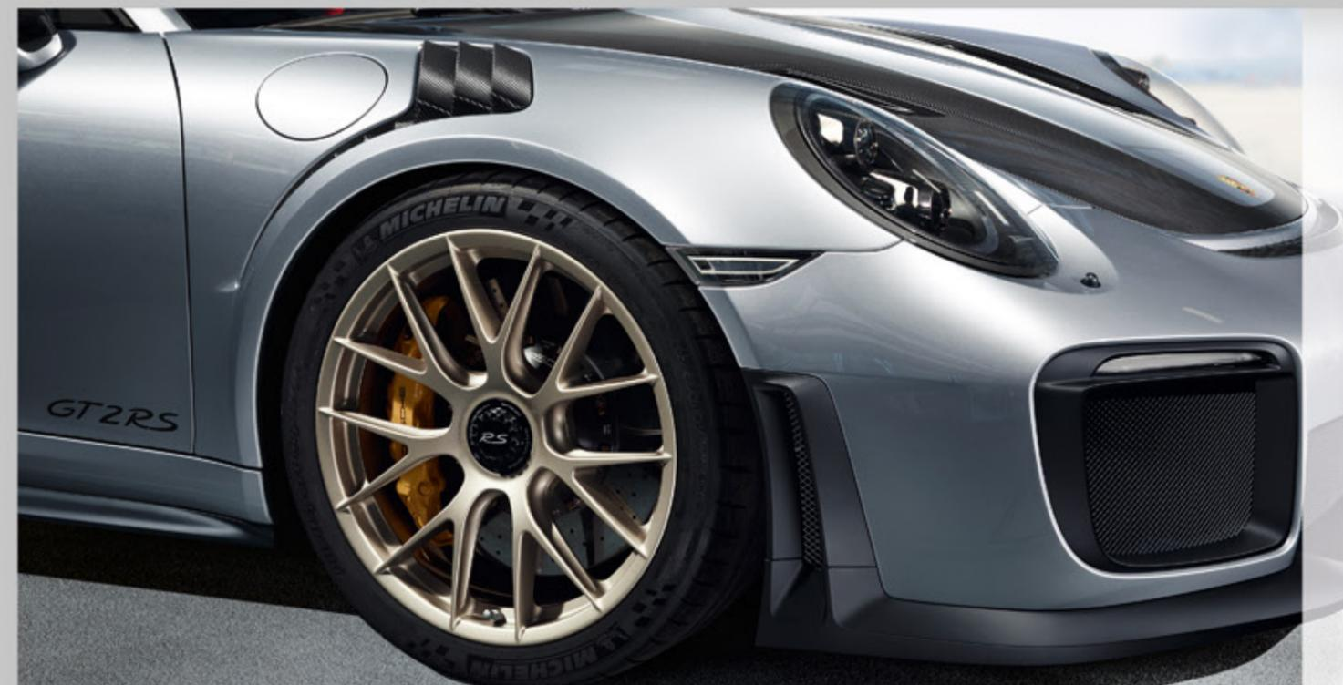
From lightweight plastic to lightweight metal. The magnesium wheels painted in satin White Gold Metallic make the new 911 GT2 RS fitted with the Weissach package approximately 11.5 kg lighter – and also enhance its visual appearance. A double victory, so to speak.
