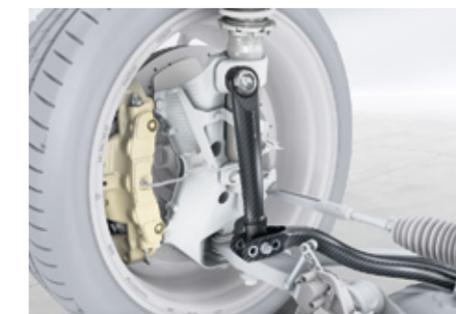
Coupling rod made of carbon
