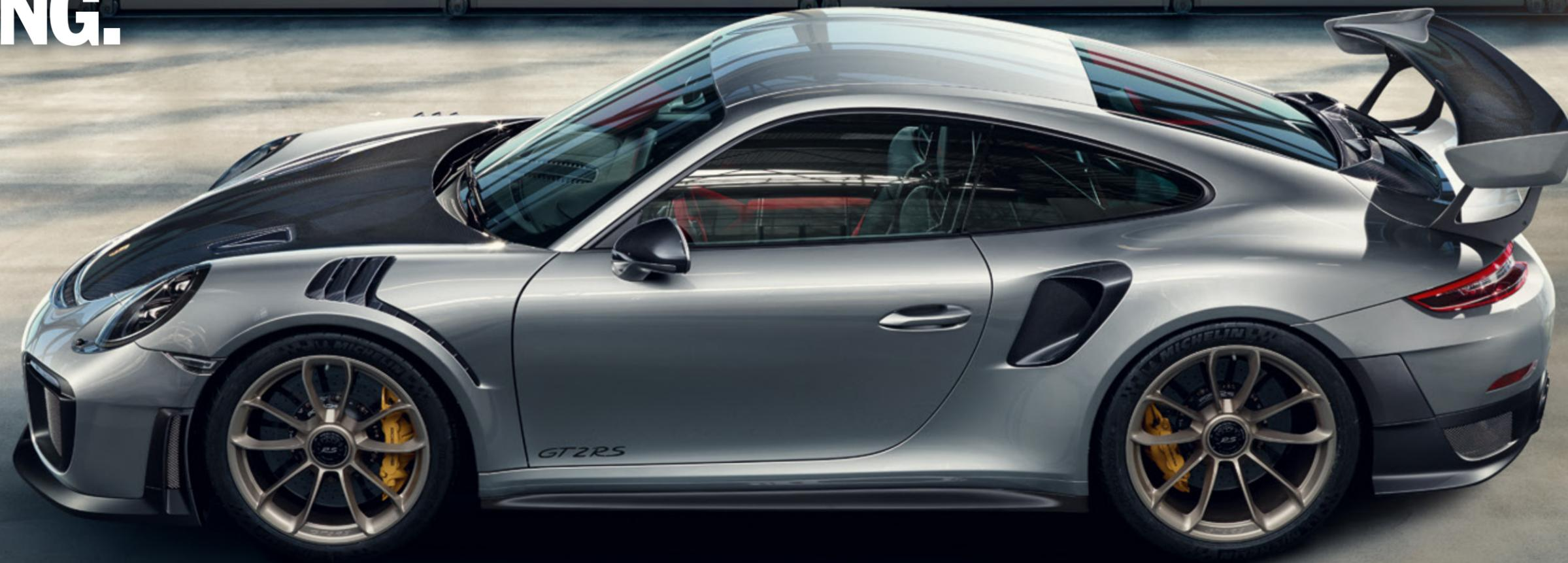
**Lightweight construction:** front lid, front wings, engine lid and rear wing made of carbon, front and rear apron made of lightweight polyurethane, rear and side windows made of lightweight glass, roof made of magnesium, rear silencers made of titanium.
