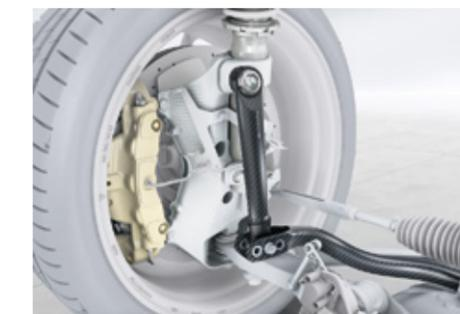
Coupling rod made of carbon
