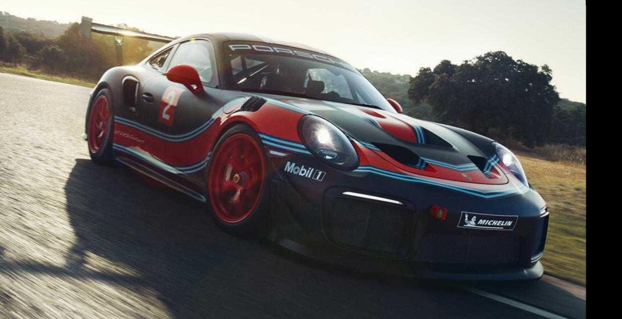
Focussing on the essentials: consistently lightweight bodywork thanks to the use of carbon-fibre reinforced plastic on the roof, front lid, front apron, doors, tail section and rear lid, as well as the elimination of any unnecessary weight in the interior. As is typical of motorsports.
