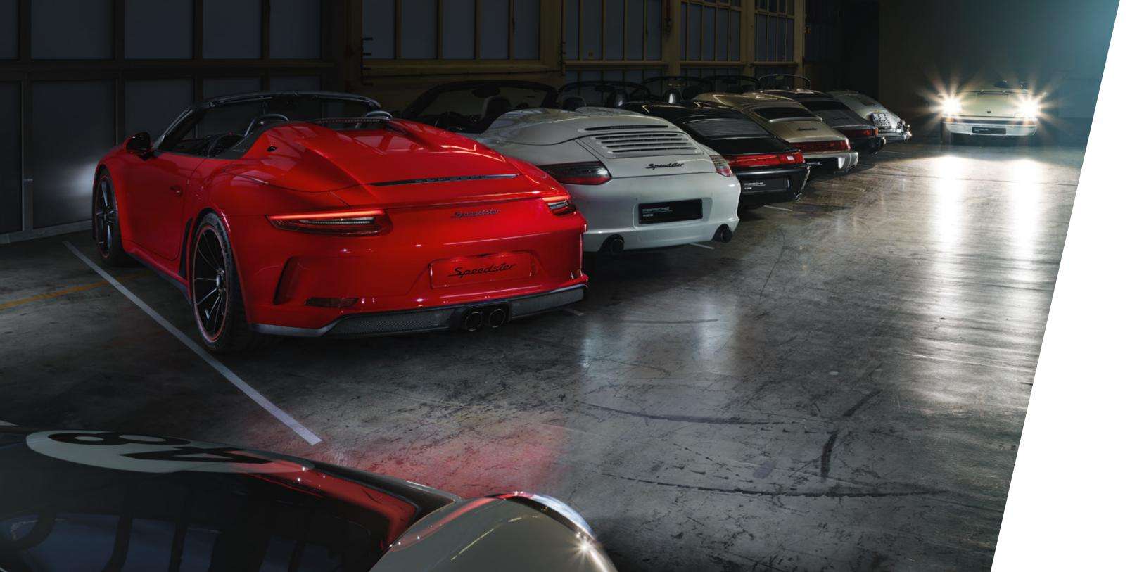
As well as a flatter silhouette, the rear view also reveals a second unmistakable feature of the Speedster: its dynamic streamliners. They are located on the rear lid which is made of carbon and moulded from a single component, making it extremely rigid.
