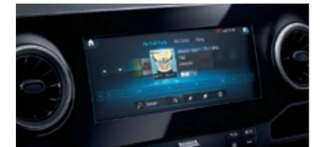
**7" AND 10.25" TOUCHSCREENS** Display screens that are activated via touch, voice control, or touch buttons on the steering wheel are available on the Sprinter.
