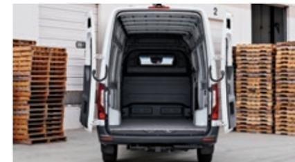
The rear doors feature hinges with self-locking mechanisms.
