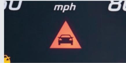
**ACTIVE BRAKE ASSIST<sup>1</sup>** This advanced system senses the likelihood of a collision with a vehicle ahead and sends both a visual and audible warning followed by initiating autonomous braking.
