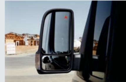
**BLIND SPOT ASSIST<sup>3</sup>** has Rear Cross-Traffic Alert (RCTA)<sup>4</sup> which employs automatic braking to avoid a collision with traffic crossing the vehicle's path (e.g., vehicles or pedestrians) when reversing.
