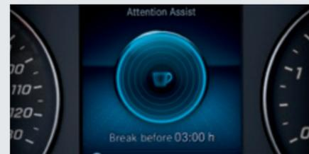
**ATTENTION ASSIST<sup>2</sup>** helps prevent drowsy driving by monitoring your driving patterns and providing an early warning in case driver fatigue is detected.
