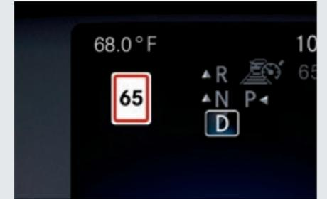
**TRAFFIC SIGN ASSIST<sup>40</sup>** uses a camera to give drivers additional help with identifying speed restriction signs, No Passing zones, and No Entry signs.
