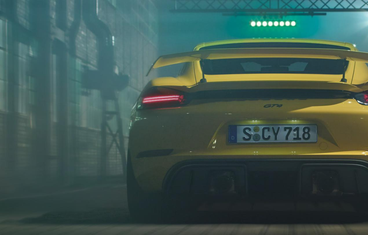
The rear is dominated by the fixed, now single-piece wing with integrated sideblades and supports in aluminum. Its racetrack origins are unmistakable, it provides downforce on the rear axle and correspondingly high traction – not just when cornering. Simultaneously, it ensures clarity and tells all optimists who want to overtake the new 718 Cayman GT4: forget it.
