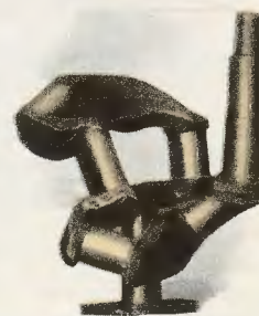
For toughness and elasticity, no better proof for Vanadium steel quality can be given than is shown in this Model T crank shaft
