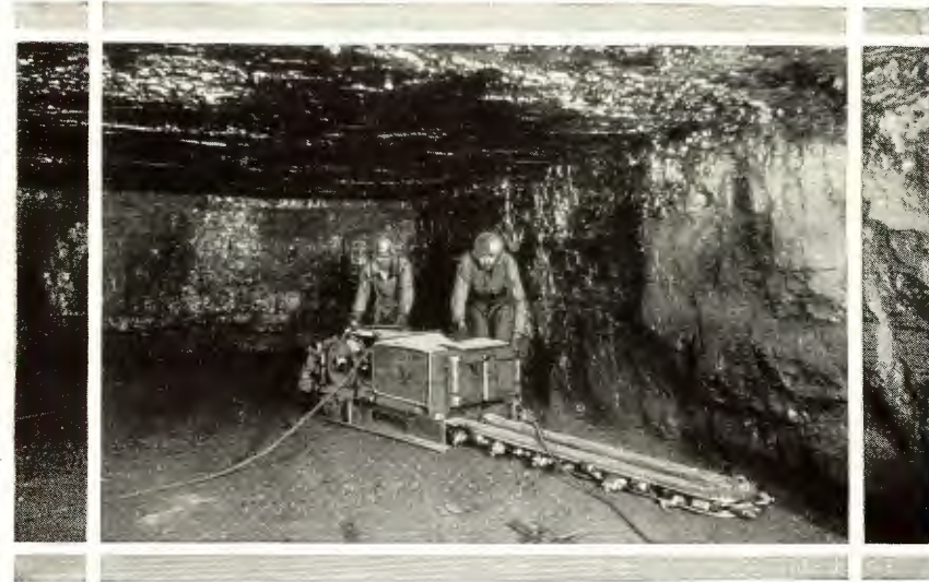
Wallins Creek Seam and Coal Cutting Machine, Interior of Coal Mine, Banner Fork Operation
