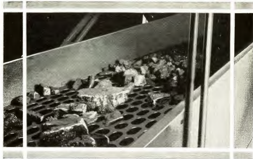
Shaker Screen for Grading Coal. Lump, Egg, Stove or Nut, and Slack Are Separated Here
