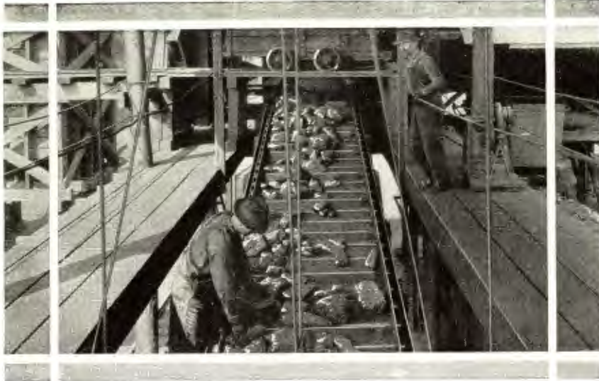
Coal on Loading Boom at Tipple; a Final Inspection and Utmost Care Against Breakage Is Given Coal in Loading
