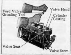
Method of grinding valve. (Cut No. 5)
