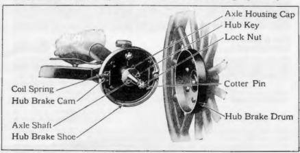
The Ford Emergency Brake. (Cut No. 15) will examine the rear axle shafts you will notice that the gears are keyed on, and held in position by a ring which is in two halves and fits in a groove in the rear axle shaft. To remove the differential gears, force them down on the shaft, that is away from the end to which they are secured, drive out the two halves of ring in the grooves in shaft with screw-driver or chisel, then force the gears off the end of the shafts.
