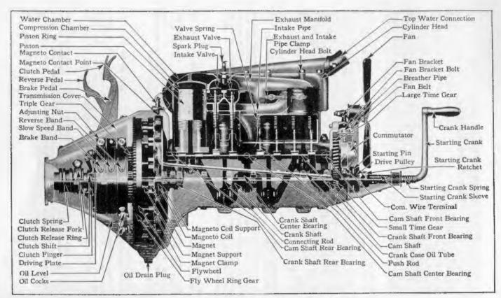
Sectional View of the Model T Motor. (Cut No. 2)
