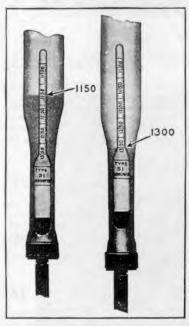
Hydrometer Readings. (Cut No. 26)
