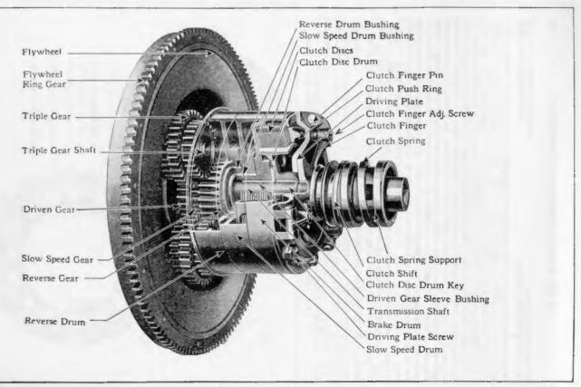
Transmission showing all gears in mesh. (Cut No. 11)
