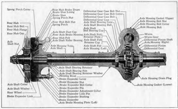
Truck Rear Axle—Longitudinal View. (Cut No. 20)
