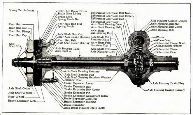
Truck Rear Axle—Longitudinal View. (Cut No. 20)
