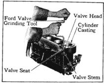
Method of grinding valve. (Cut No. 5)
