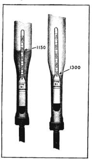
Hydrometer Readings. (Cut No. 26)
