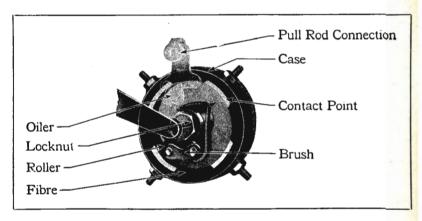
connected with a coil unit, an electrical circuit is passed through the entire system of primary wires. This circuit is only momentary, however, as the roller passes over the contact point very rapidly and sets up the circuit in each unit as the roller touches the contact point connected with that unit. The commutator should be kept clean and well oiled at all times.
