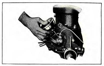
Oiling the Ford Commutator. (Cut No. 19)
