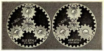
Fig. 397 Correct Assembly
