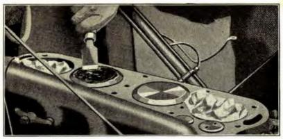
and valves are clean. With the end of a small screw driver, loosen any dirt or carbon in the bottom of the cylinder head bolt holes and blow out the carbon with compressed air. This is done to permit cylinder head bolts being drawn down tightly and eliminate the possibility of water and compression leakage after cylinder head is installed.
