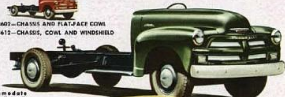
MODEL 3603—CHASSIS AND CAB Accommodates bodies 72" to 92". Weight of body and payload, up to 3100 pounds
