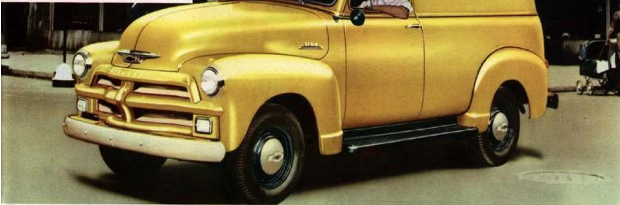
MODEL 3105 PANEL 116" WHEELBASE, MAXIMUM G.V.W. 4800 LB.
