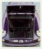
The space-saving front axle takes up so little room in front that a very large 200-liter (7.1 cubic foot) trunk is possible.
