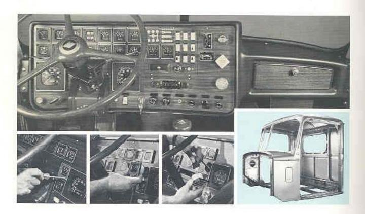
Maximum convenience for the driver and the mechanic. Note these bold instruments, a Diamond Reo exclusive sure to rate with both the fleet owner and the individual operator. Readability. Tops! The fire orange indicator is easy to read against a black field and the warning lamp is located within the gauge where it belongs. Any hazard condition is immediately pinpointed. All instruments are located in strict compliance with RCGC/SAE recommendations.
