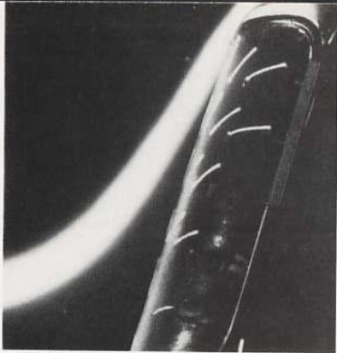
Cab design creates a laminar (streamlined) airflow over cab profile.
