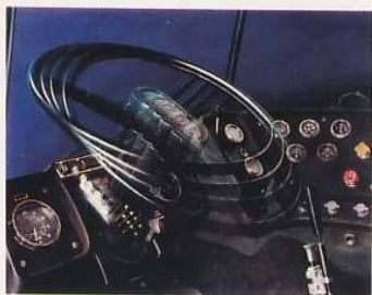
Standard tilt steering column adjusts to driver preference through a 12° arc and provides a 64° flat wheel position for added leverage in close-quarter maneuvering.
