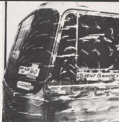
Cab corner radius and sloped windshield help reduce side splash.
