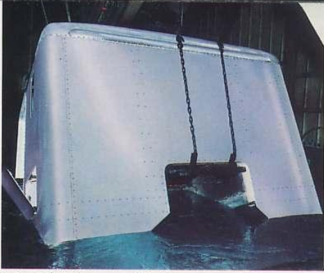
Every cab is immersed in Elpo emulsion
