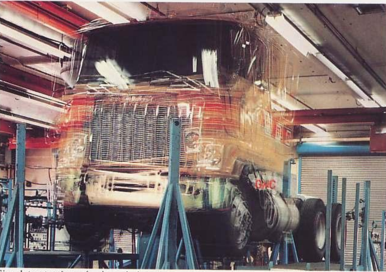
Simulator testing of cab and chassis components
