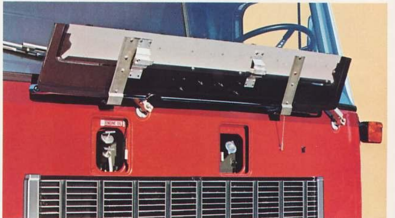
Cab-front door for access for oil and coolant service
