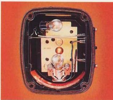
Shock-mounted rear lamps
