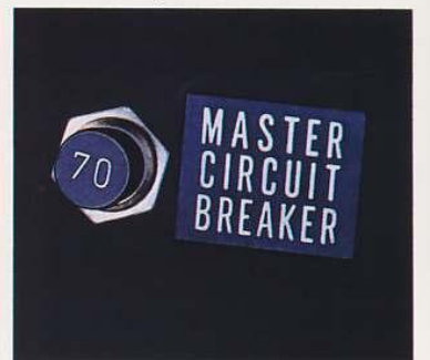
70-amp master circuit breaker
