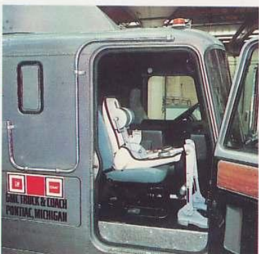
Simulator tests duplicates in weeks punishment on springs and seats that will be sustained in years of actual operation.
