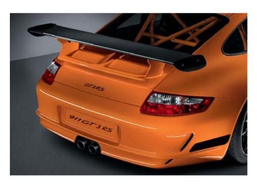
The rear wing on the 911 GT3 RS is derived from the 911 GT3 Cup racing cars. Made from genuine carbon fibre, it is not only lighter than the wing on the 911 GT3, it has a larger surface area producing additional downforce. The wing is adjustable on both models and provides greater stability at high speed.
