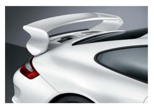
The most prominent feature at the rear of the car is the fixed bi-plane wing structure. The angle of incidence on the upper wing element can be adjusted for racing use. It also offers even greater stability at high speed. An interesting detail on the lower wing surface is the smaller rubber spoiler or 'Gurney flap'. This device creates additional downforce with a negligible increase in drag.
