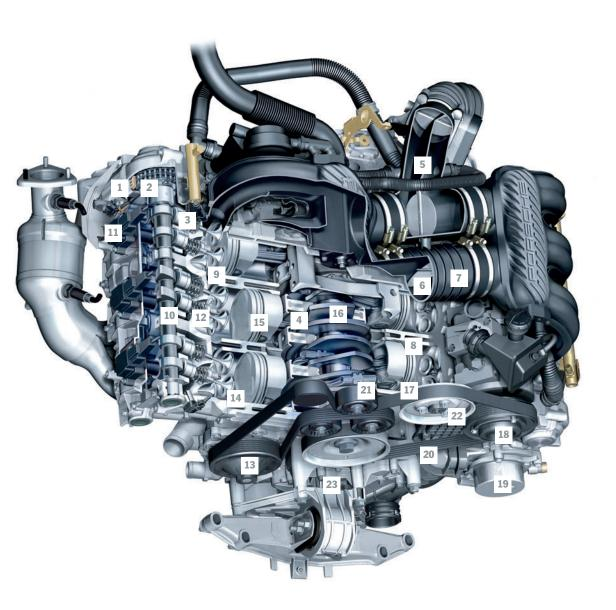
This illustration identifies key components of the Boxster's namesake six-cylinder boxer engine. It's called "boxer" because the power plant's horizontal layout places the pistons in direct opposition, creating a "punch-counterpunch" effect with each rotation of the crankshaft.
