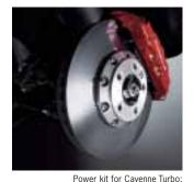
380 mm two-piece brake disc on the front axle
