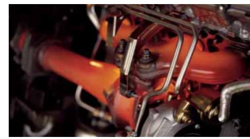
Cayenne turbocharged engine, turbocharger
