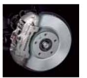
Standard brakes on Cayenne S: 350 mm disc brake on the front axle
