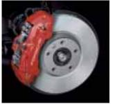
Standard brakes on Cayenne Turbo: 350 mm disc brake on the front axle
