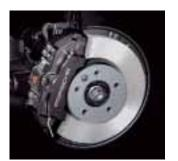
Standard brakes on Cayenne: 330 mm disc brake on the front axle
