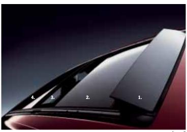
The forward segment (marked 1 in the illustrations above) lifts upwards (figure 2) to act as a wind deflector, minimising noise and turbulence even at high speeds.
