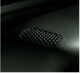
AudioPilot system microphone mounted left of the steering column to monitor interior noise level
