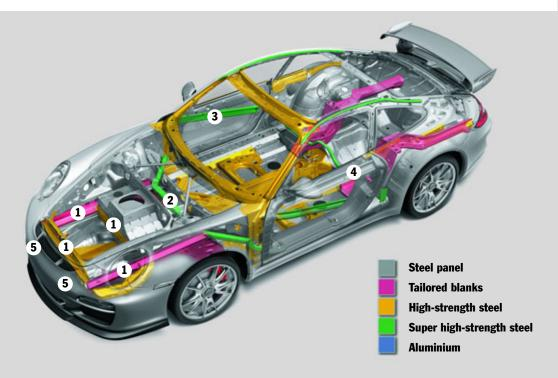
channel energy into the side structure and thus further protect the passenger cell. In the event of a minor collision, a system of easily replaceable impact absorbers (5) prevents more serious damage.
