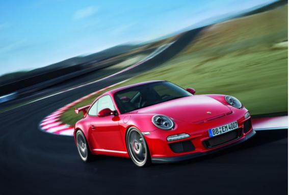
The wheel dimensions are 8.5J x 19 with 235/35 ZR 19 tyres (front) and 12J x 19 with 305/30 ZR 19 tyres (rear). Road-legal sport tyres provide the necessary grip, although the lower tread profile presents a greater risk of aquaplaning on wet roads.
