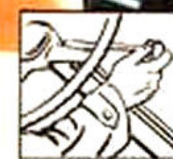
Steering column control with 3-speed transmission
