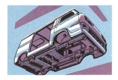
**GALVANIZED PROTECTION** against rust and corrosion for longer body life. All main underbody structural members on the Econoline Van are heavily zinc-coated to resist rust, for greater durability.
