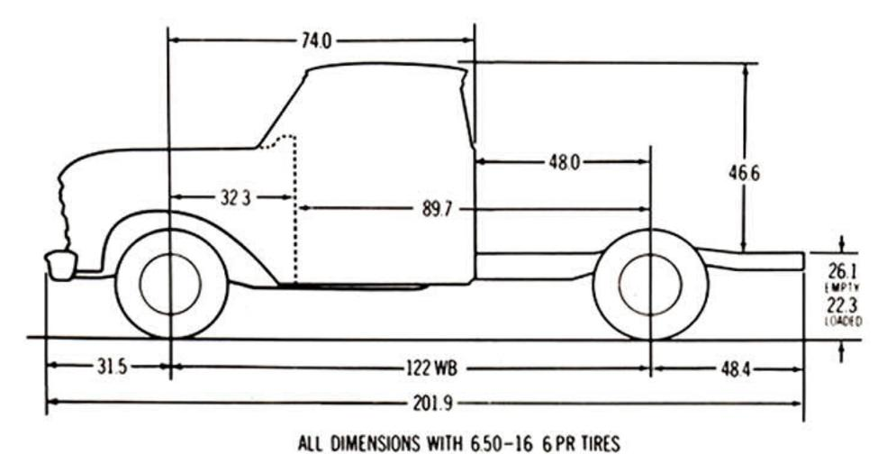
Chassis-Cab, Chassis-Cowl — Ford's F-250 chassis models are especially suited for custom-built bodies from 7 to 8 feet long. The Chassis-Cab models are available for special-purpose bodies available from any number of independent body builders. Chassis-Cowl and Chassis-Windshield units may be easily converted to single-unit bodies of the walk-in type.
