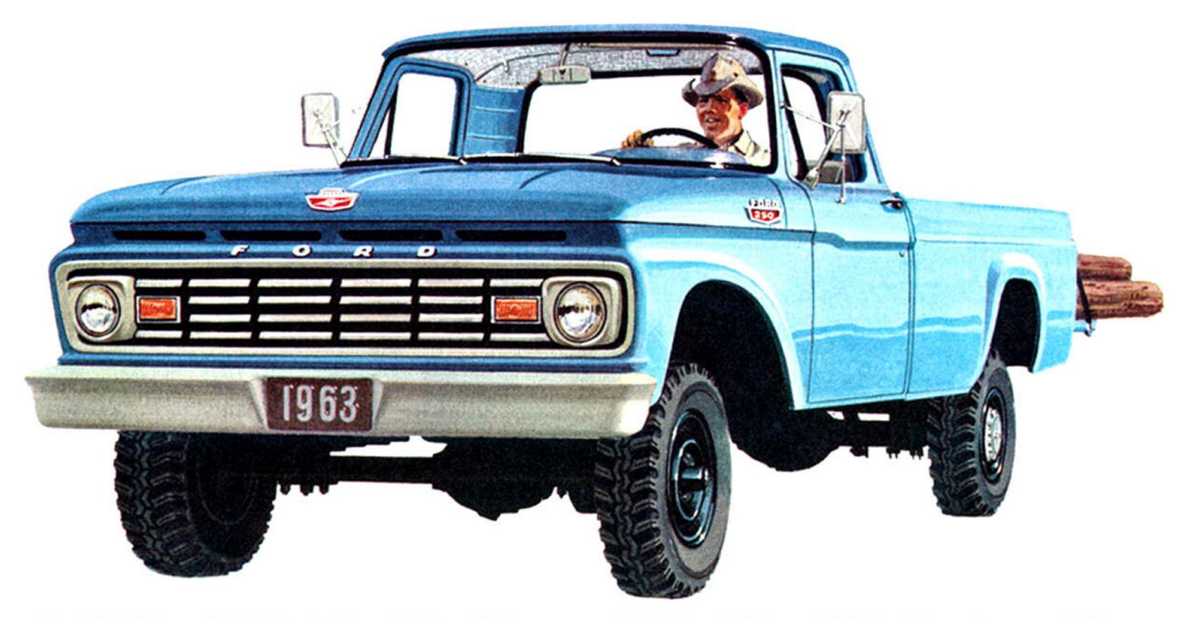
Ford F-100 and F-250 4-Wheel Drive Pickups have the power and extra traction needed for severe off-road work. For '63, Ford 4 x 4 units are built to provide more driver comfort, more operating reliability, and more durability. They're built like big trucks with such features as deep-channel parallel-rail frames, two-stage rear leaf springs, optional auxiliary springs (F-250), and short-stroke engines.
