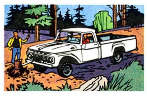
Front-mounted PTO-driven winches, pumps, scoops, snow blades, sweepers, etc., combined with 4 x 4 mobile power, make light work of tough jobs. Engine power is transmitted to do the job easier and faster.
