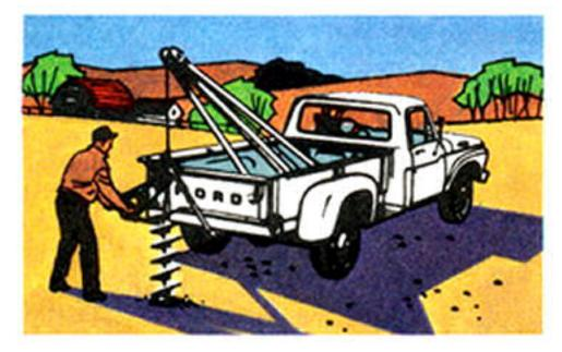
Rear-mounted PTO-driven mobile worksavers, such as post hole diggers, feed mills, saw mills, hay balers, power lift tailgates and many other gear, belt or hydraulically actuated units are easily installed.
