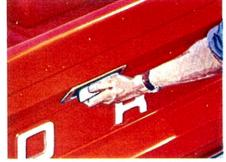
NEW ONE HAND TAILGATE New, easy, one-hand tailgate latch gives greater loading ease and the husky support straps disconnect easily allowing a straight down tailgate position.
