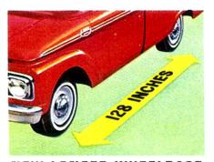
NEW LONGER WHEELBASE The new 128" wheelbase (6" longer) will give you a smoother ride, better weight distribution and top stability under all load and road conditions.
