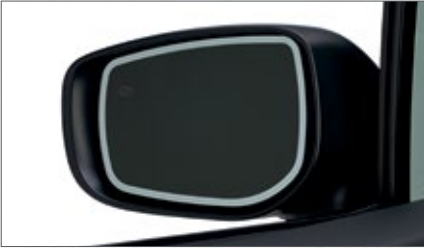
Auto-Dimming Exterior Mirrors with Approach Light. Enhance nighttime driving safety by adding these mirrors. Upon approaching the vehicle or unlocking your doors with the keyless entry system, LED lights located behind the Subaru logo in each exterior mirror will illuminate the ground next to and towards the rear of the vehicle. During nighttime driving, the Auto-Dimming Exterior Mirrors will reduce headlight glare by dimming in unison with the Auto-Dimming (Interior) Mirror. Dimming level is regulated by the level of light detected from the Auto-Dimming (Interior) Mirror. Requires Auto-Dimming (Interior) Mirror.
